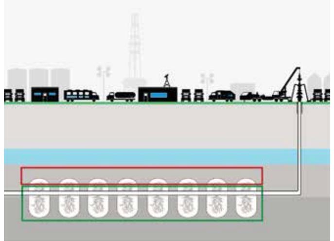
With conventional shaped charge technology (diagram upper right) casing entry hole size variation leads to non-uniform frac clusters. This frequently results in inadequate access to the upper portion of the pay zone and reduced production potential.
