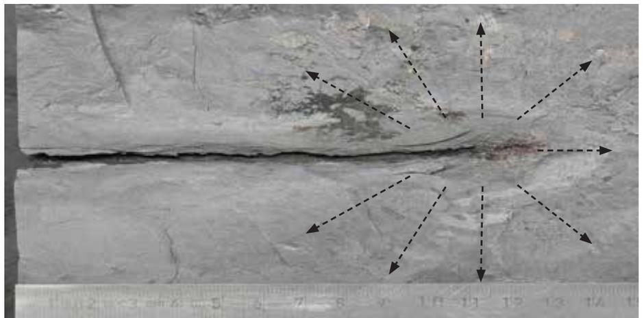
HALOFRAC PERFORATION TUNNEL IN SHALE
