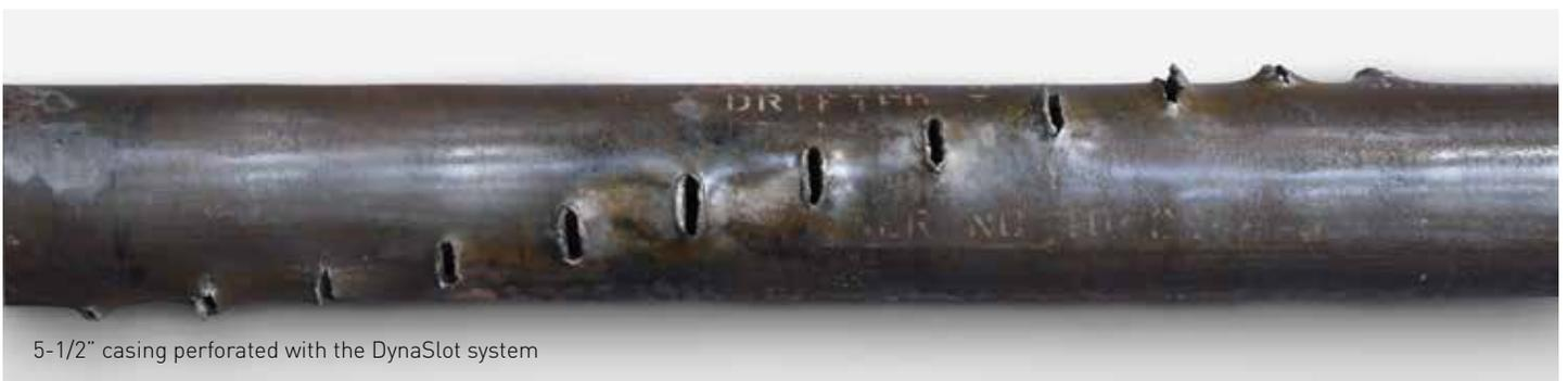
5-1/2" casing perforated with the DynaSlot system
